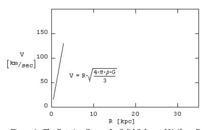
Figure 4 - The Rotation Curve of a Solid Sphere of Uniform Density
