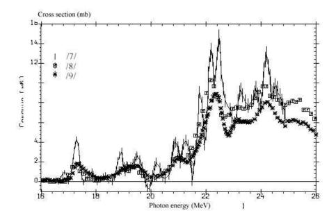
Figure 1: The comparison of photoneutron cross sections  ${}^{16}O(\gamma, xn)$  obtained in one BR-experiment (Moscow State University) and two QMA experiments carried out at Saclay (France) Livermoore (USA). Figure is taken from [18] where also references to experiments can be found.
