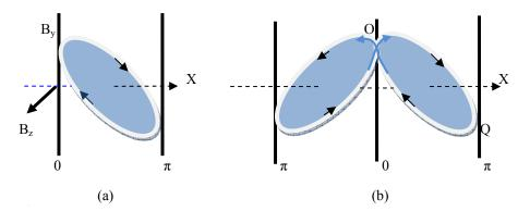
(a) This represents the standing helical half wave formed between two reflecting mirror.
