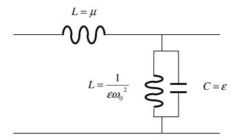
The transmission line is dispersive because the characteristic impedance (29) is frequency dependent and it resonates when:
