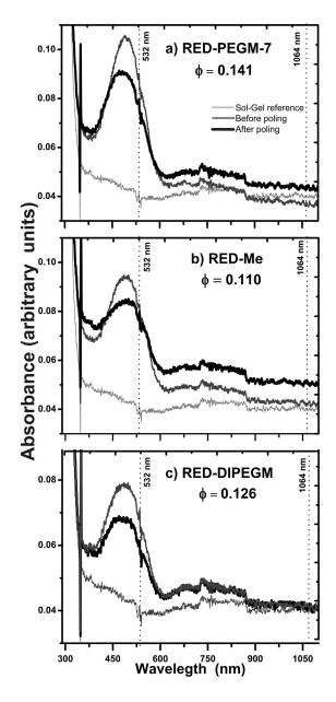
FIGURE 4. Comparative UV–Vis absorption spectra of the pure sonogel reference and the hybrid film samples, before and after performing electrical poling: a) RED-PEGM-7 based hybrid film, b) RED-ME based hybrid film, and c) RED-DIPEGM based hybrid film.
