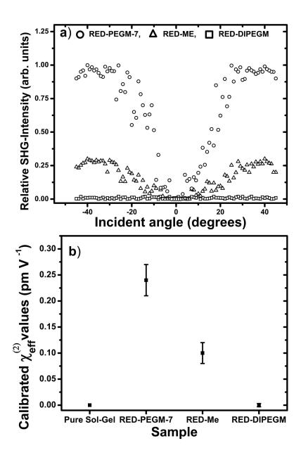
FIGURE 5. SHG/NLO-measurements performed on the hybrid thin films according to the Maker-Fringes technique: (a) angle dependent SHG measurements (P-In/P-Out polarizing geometry) and (b) calibrated NLO-coefficients.
