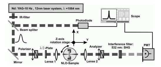
FIGURE 2. Experimental set-up for SHG measurements in hybrid thin films. 150x62mm (600 x 600 DPI)
