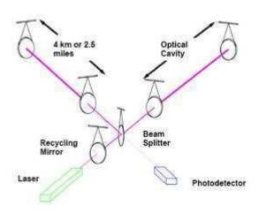
Fig. 5 Schematic diagram of Laser Interferometer Gravitational-wave Observatory
