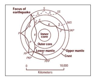
Fig. 2 Cross section of the whole Earth, showing the complexity of paths of earthquake waves. The paths curve because the different rock types found at different depths change the speed at which the waves travel. Solid lines marked P are compressional waves; dashed lines marked S are shear waves. S waves do not travel through the core but may be converted to compressional waves (marked K) on entering the core (PKP, SKS). Waves may be reflected at the surface (PP, PPP, SS).
