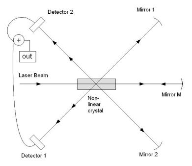
**Fig. 5**: Scheme of interferometric antenna for detection of gravitational wave in the  $\oplus$  polarization in which a linear crystal splits the incident beam in two ones forth and back.
