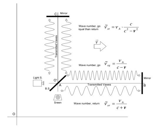
Figure 6: Michelson-Morley experiment setup and representation of transmitted wave number in each two way light path.
