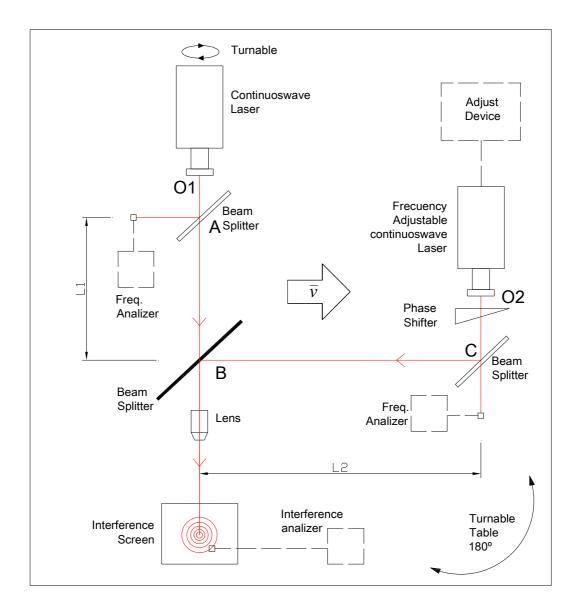
Figure 9: Schematic of the proposed experimental set-up for checking the anisotropy of c with perpendicular beam compare.
