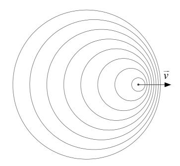
Figure 1: Classical representation of the wave fronts transmitted to a static medium by a moving emitter. For a static observer the transmitted frequency is anisotropic but not the wave speed.
