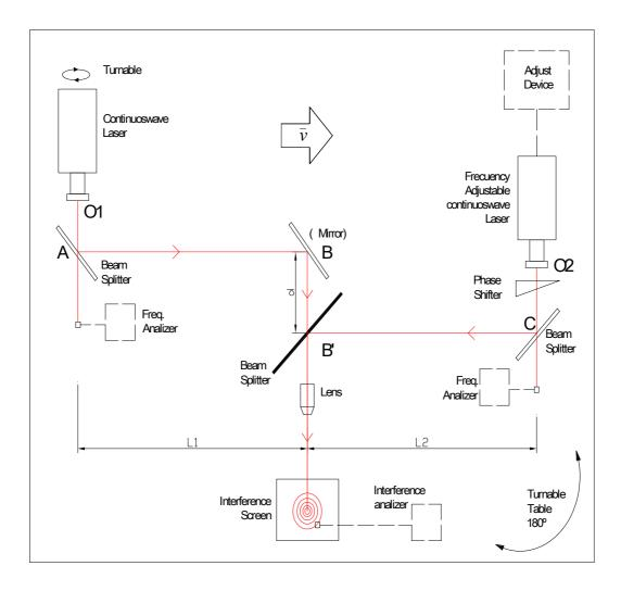
Figure 8: Schematic of proposed experimental set-up for checking the anisotropy of c with linear beam compare.
