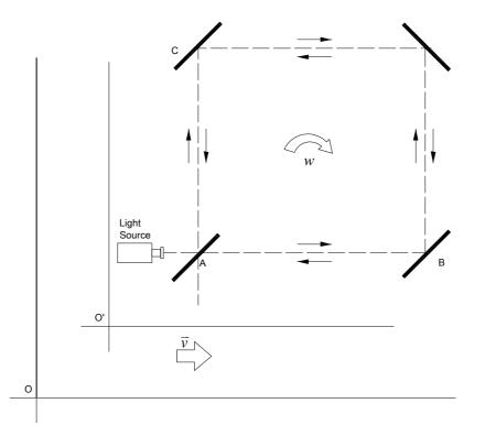
Figure 7: Schematic of the Sagnac experiment aimed to detect the ether by rotating opposite paths from the same light source.
