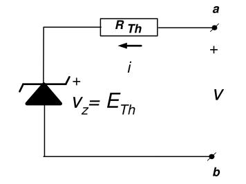
This is the partial (not for any sign[i]), **passive mode** equivalence that is important for creation of nonlinear resistors v(i), see Slide 11.
