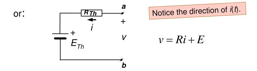
**This case** of *i* entering the circuit (and sign[i(t)] = const) is <u>equivalent</u> to the following **obviously nonlinear** circuit:
