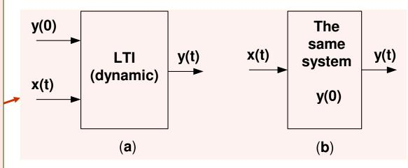
Notice that in the domain of the Laplace variable, the interpretation of the initial values of state variables as "inputs" is even a standard one.
