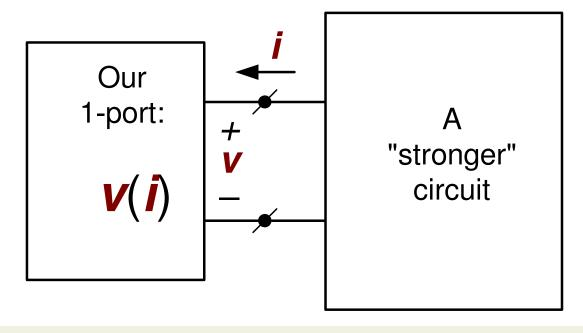
A 1-port is used for creation of a nonlinear resistor
