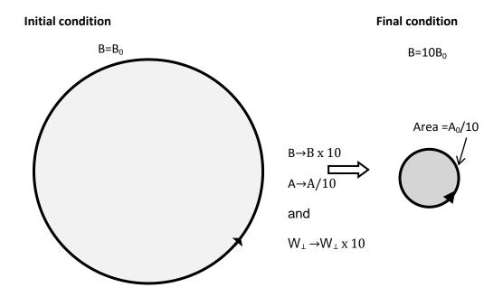
For a uniform magnetic field, B, at right angles to the area, A, the magnetic flux,  $\Phi$ , is given by:  $\Phi = B A$
