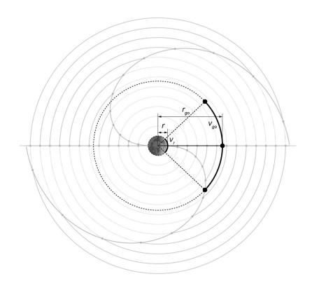
*Figure 2.1.1.c* Geostationary orbit as a second class lever. Both radiuses r and r<sub>go</sub> represent legs, i.e. distances from its fulcrum.
