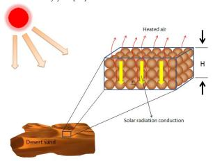
Fig.6 A model of heat exchange system in desert sands under the sun's radiation. H represents the depth that the sun's radiation is conducted into desert sands. r represents the radius of sand particle.
