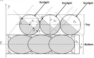
Fig.4 Illustration of solar irradiation of spherical sand particles in a rectangular plane. The white regions represent the area irradiated by sunlight, grey regions are shaded areas that cannot receive sunlight; r denotes the radius of the spheres; Top: the surface layer of particles. Bottom: the projection of the surface layer of particles immediately on the plane. The values  $S_3$  to  $S_8$  represent illuminated areas (see the text for details).
