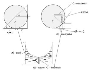
Fig. 5 Illustration of calculations of the area irradiated on the plane by sunlight that passes the first row of spheres (the spheres at the right of Figure 3, which have an illuminated area  $S_3$  in Figure 4). The region covered by short black lines denotes the irradiated area on the plane.
