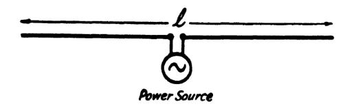
The movement of air particles in the tubes and of the electrons the antenna is oscillatory: they move forwards-backwards (to-and-fro) along the antenna about fixed positions executing simple harmonic motions.
