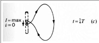
and at a  $\frac{1}{4}$ -period they pass at the midpoint (Fig. 2-22c). As this happens, the field lines detach and new ones of opposite sign are formed. At this time the equivalent current I is a maximum and the charge acceleration is zero.
