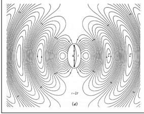
Five stages of radiation from a dipole antenna are shown in
