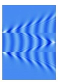
After a few oscillations a number of wavefronts moving in directions approximately perpendicular to the direction of the antenna are formed; the distance between two of wavefronts is the wavelength  $\lambda$  of the radio wave emitted:
