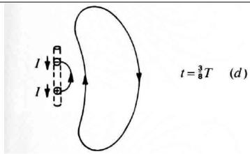
As time progresses to a  $\frac{1}{2}$ -period, the fields continue to move out as in Fig. 2-22d and e.
