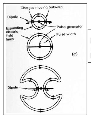
At the next stage [(a) middle] the charges reach the ends of the dipole, are reflected (bounce back) and move inward toward the generator [(a) bottom].
