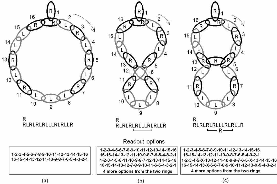
**Fig. 3.** Example of compound from entangled photon loops. Below each compound the notation for interconnections are shown. The corresponding readout options are shown in the boxes at the bottom: (a) – a simple compound loop where the loop R indicated the beginning of the encoded word; (b) – a compound loop with an internally connection of 0-order; (c) – a compound loop with an internal connection of 1<sup>st</sup> order.
