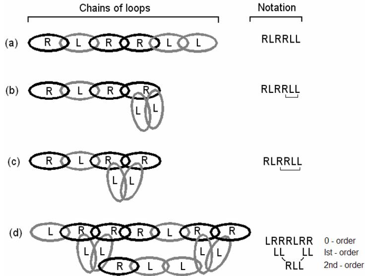
**Fig.2.** Interconnected chains of loops. (a), (b) and (c) – illustrate different connection; (d) illustrated connections of different order
