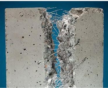
This is fiberglass in concrete. This is the same structural idea with which carbon strengthens iron to make steel.
