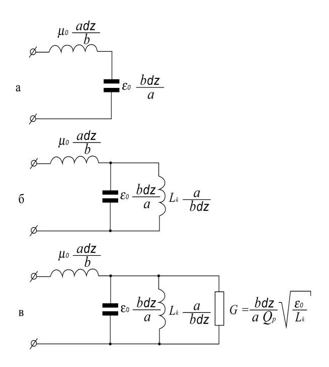
Fig. 2. a - the equivalent the schematic of the section of two-wire circuit; b - the equivalent the schematic of the section of the two-wire circuit, filled with plasma without the losses; B - the equivalent the schematic of the section of the two-wire circuit, filled with the plasma, in which there are ohmic losses.
