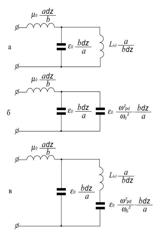
Fig. 7. Equivalent circuit of two-conductor line segment with a dielectric: a -  $\omega \gg \omega_0$ ;  $\delta - \omega \ll \omega_0$ ; B – the whole frequency range.
