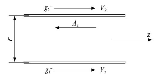
Fig. 1. Schematic view of force interaction between current-carreging conductors of a two-conductor line in terms of the present-day model.
