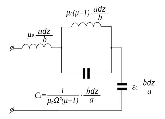
Рис. 8. Equivalent circuit of two-conductor line including a magnet.
