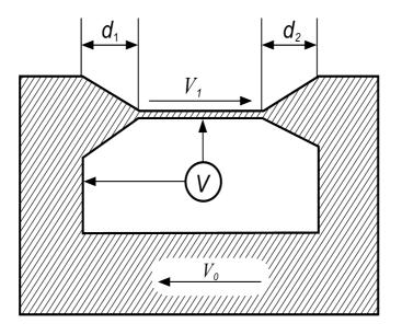
Fig. 3. Schematic view of a current-carrying circuit based on a superconducting film.
