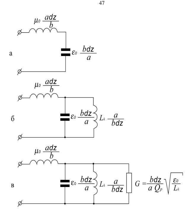
Fig. 6. a. Equivalent circuit of the two-conductor line segment;
