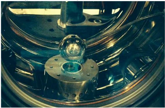
A vacuum chamber with a marble-size sphere at its center was used to test the nature of dark energy.
