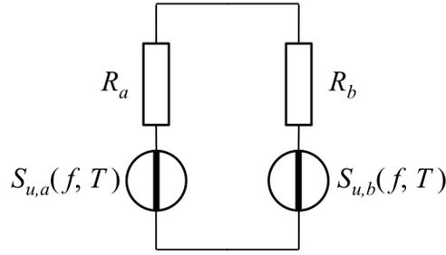
Figure 1. The second law of thermodynamics requires that the net power flow between resistors  $R_a$  and  $R_b$  is zero. This is provided by the functional form of the power density spectrum  $S_u(f, T)$  of Johnson noise (represented by voltage generators in the figure), which is, at any frequency and temperature, proportional to the resistance.
