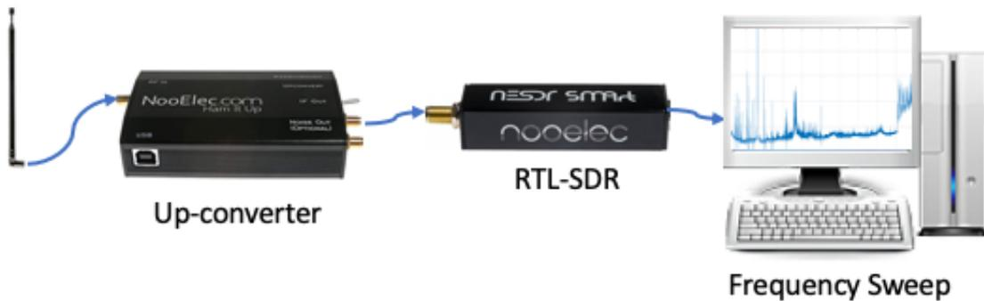
Figure 10 Radio Receiver
