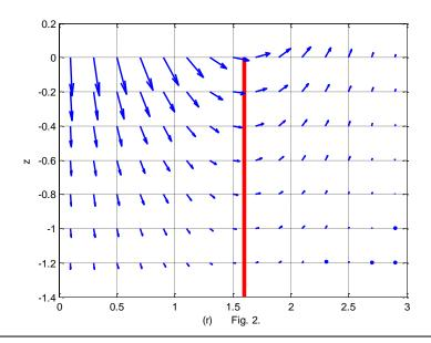
So, there exists a certain radius of "vertical calm" for which the vertical flow of water is not present  $(J_z = 0)$ , and more close to the center of whirlpool the water flow is directed down  $(J_z < 0)$ , but with increasing distance from this radius the water begins to rise  $(J_z > 0)$ . And so the water of surrounding ocean pours into the funnel with this radius of "vertical calm".
