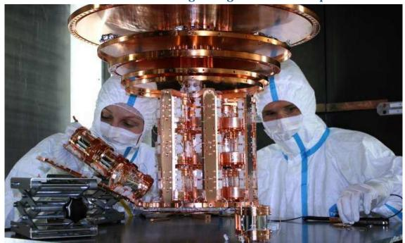
By carefully re-engineering a detector for heavy dark matter particles, so-called WIMPS, the CRESST collaboration succeeded in improving the detector to measure lightweight dark matter particles with masses in the range of a proton mass. Credit: Max Planck Institute for Physics
