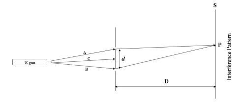
Fig.1. Schematic diagram for the double slit experiment with electrons: An
