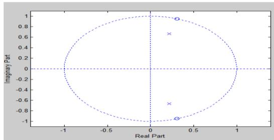
Figure 2 Poles and Zeros of the Notch Filter
