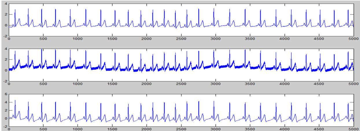
Figure 7 Application of Notch DC Notch filter to ECG with PLI and Baseline
