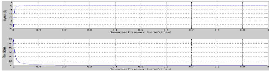
Figure 5 DC Notch Filter Characteristics
