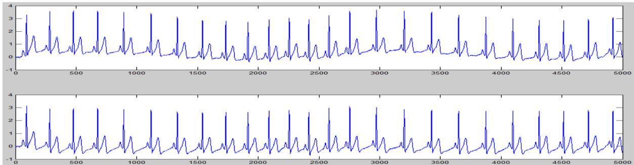
Figure 6 Application of DC Notch filter to ECG with Baseline
