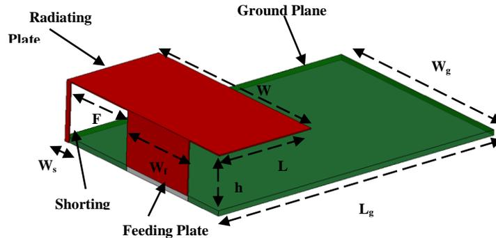
Fig. 1. The Geometry of the studied PIFA antenna
