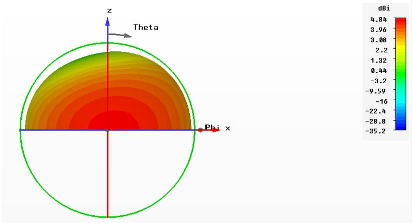
Fig. 3. The radiation pattern for the proposed antenna without head
