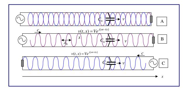
In the picture above (picture A) a transmission line is connected to a sinusoidal voltage source. the transmission line is terminated with an adequate resistor . and a standing wave is created along the transmission line. It was proved that a standing wave is a superposition of two waves moving in opposite directions, each wave with velocity c. So instead of one Transmission-line I use two. One for the wave going
