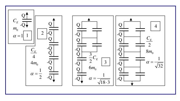
Suppose all the capacitors in the picture above are the same. In case [2] the charge between two capacitors is induced charge. The equivalent capacitance of 4 capacitors
