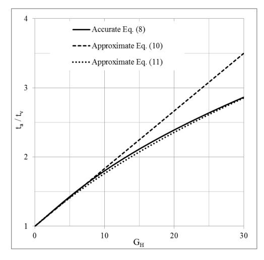
FIG. 1. The free-fall time in air calculated using the accurate equation (8) and two approximate equations (10) and (11).
