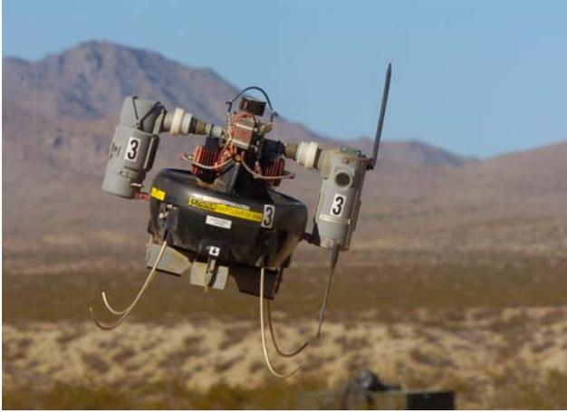
The Honeywell RQ-16 T-Hawk, Micro Air Vehicle (MAV), flies over a simulated combat area
