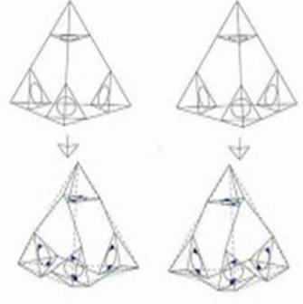
Space fill unit with RIGHT hand rotation.      Space fill unit with LEFT hand rotation.
