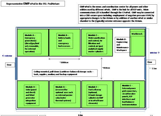
Figure 14 - EMP – Electro-Mechanical-Power (Energy) Pod
