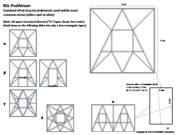
Figure 8 – Fundamental nPod Frame Element Panel – Alpha Config
