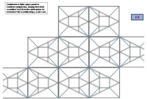
Figure 10 - Combining Alpha and Cantilever elements for large multi-level PodAtriums
