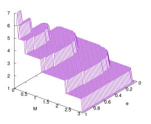
FIG. 2. The number of iterations needed for a relative accuracy of  $10^{-12}$  in *E* starting from (12) iterating with (8).
