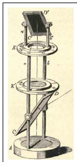
shown in the left figure [5], which is a variation of Biot's original polarizing apparatus, shown at right [6]. In both cases, a beam of light is reflected by one glass plate onto a second glass plate, as explained above.
