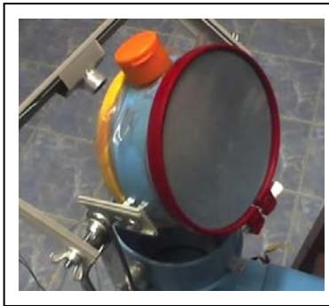
Each acoustic plate is therefore like a 50 mm thick disk, or drum, having two parallel surfaces of thin elastic membranes that separate the interior of the plate from the exterior (left picture).
