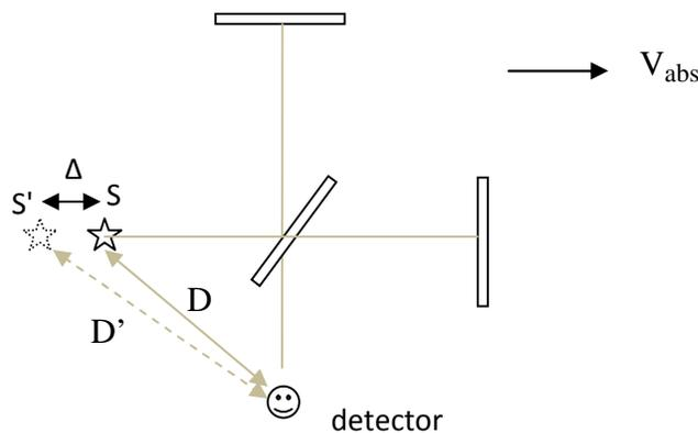
From the above diagram of the Michelson-Morley experiment, we see that the effect of absolute velocity is just to create an *apparent* change of the position of the light source *relative* to the detector. The apparent change in position is determined by the direct source-detector distance  $D$ , the orientation of the source-detector line with respect to the absolute velocity and the magnitude of the absolute velocity[1].
