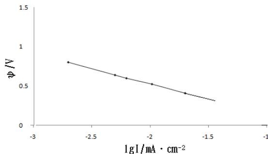
Fig.2 Cathodic polarization curve of electrolytic process
