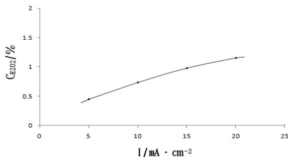
Fig.3 Concentration change of hydrogen peroxide increasing with current density
