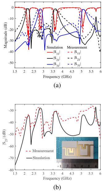
Fig. 5: Simulated and measured responses of the quad-channel diplexer (a) Transmission and reflection coefficient, (b) Isolation and photograph
