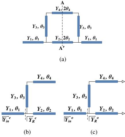
Fig. 3: Equivalent circuits of the (a) QMSRR in (b) Even-mode and (c) Odd-mode.
