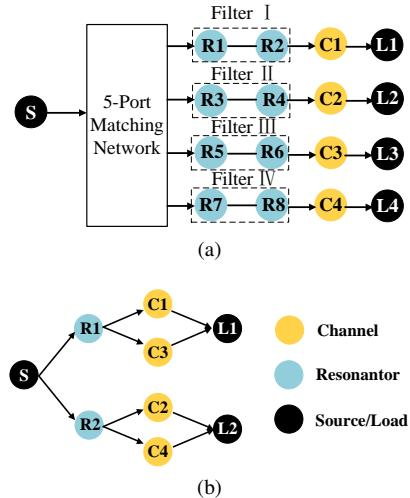
Fig. 1: coupling scheme of a quad-channel diplexer. (a)Conventional structure. (b) Proposed structure.
