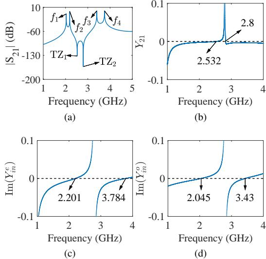
Fig. 4: QMSRR (a) Frequency response of the QMSRR with weak coupling (b) Transmission zeros (c) Even-mode resonant frequencies and (d) Odd-mode resonant frequencies.
