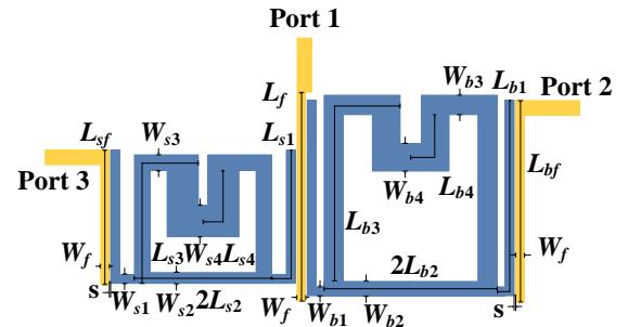
Fig. 2: Layout of the proposed quad-channel diplexer.
