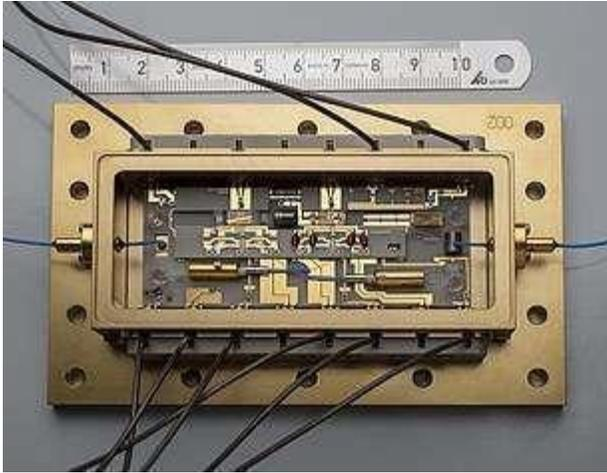
A micro-integrated diode laser module (ECDL-MOPA) from the Ferdinand-Braun-Institut emitting at a wavelength of 1064 nm. Credit: FBH/schurian.com
