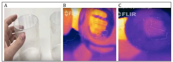
Figure 17. Thermal Imaging camera Greenhouse gas demonstration. (A), two glasses, one fill with air (mostly N2 and O2) and the other with a GHG, presumably CO2; (B), the first glass is non-thermoelectric, wrongly said to be 'transparent to IR'; and C, the GHG is thermoelectric, wrongly said to be opaque to IR. [47]
