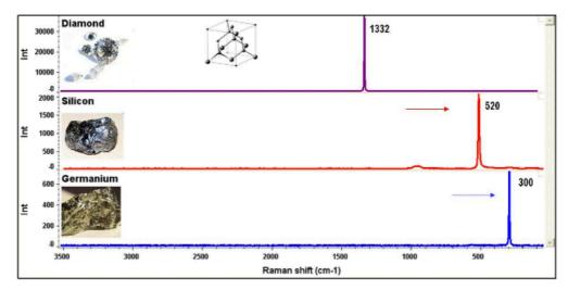
Figure 1: Raman spectra of diamond, crystalline silicon, and crystalline germanium
