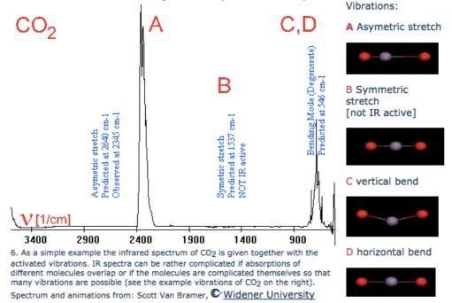
**Figure 10.** CO<sub>2</sub> Thermoelectric IR Spectra. A 'negative' image of the above image (Figure 32) showing CO<sub>2</sub>'s IR active electric dipole vibrational modes and one non-IR active. [51] 1538 cm<sup>-1</sup> clearly shown absent; incorrectly indicated as 'not IR active' when it is more correctly non-thermoelectric due to symmetric stretch.
