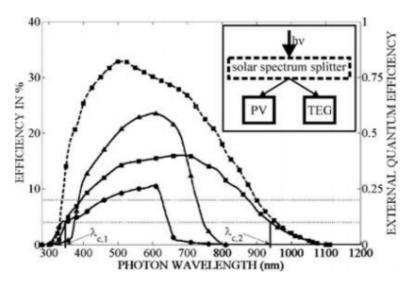
FIG. 2. Schematic diagram of the PV-TE hybrid system. EQE (dashed line) and spectral conversion efficiency (solid lines) of a-Si:H (▲), mc-Si:H (■), and polymer (●), assumed solar TEG efficiency of 4% and 8% (dotted lines).
