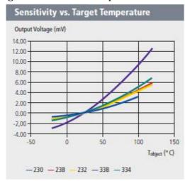
Figure 4. Thermopile Voltage output by Temperature
