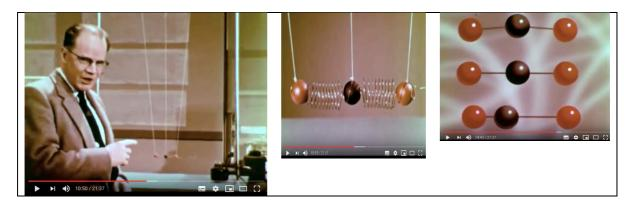
**Figure 46. Demonstration of Harmonic Vibration of** <u>all</u> **of CO2's Modes.** Frame A, a model the CO2 molecule is vibrated by frequency producer at different frequencies; frame B, close up of the spring and ball model attached to the devise on the right; and Frame C, the film showing – in an age before Raman Spectroscopy – all CO2's modes and their positions.
