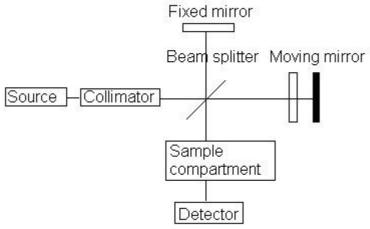
Figure 6. Operations Schematic of Fourier Transform IR (FTIR) spectrometer [20]. 3.4.3 Spectroscopy Beer-Lambert Law
