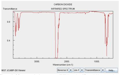
**Figure 9. CO<sub>2</sub> transmission spectra. [28]** Here the differential between the reference 1500°C heat source and the ambient temperature CO<sub>2</sub> gas is clearly shown. Predicted absorption bands are shown, however, this indication would decrease if the temperature of the CO<sub>2</sub> were equal to the reference heat source.
