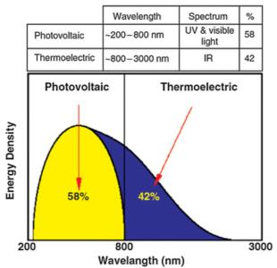
Figure 24. Simplified solar spectrum and energy ratios to be used within the PV cell and the TEG [56]. This schematic shows a shape and profile similar to the IR generated Solar irradiance spectrum – by no coincidence.
