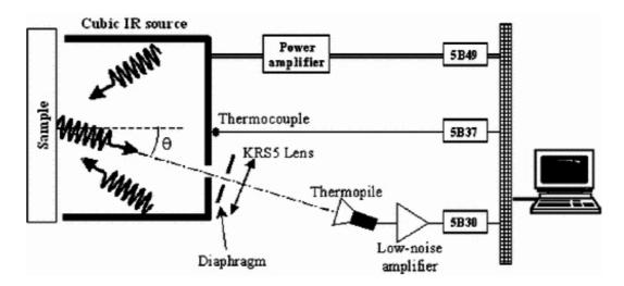
**Figure 22 Measurement of Emissivity.** The emissivity is measured by the thermocouple for it real temperature and by the thermopile (for its heat radiation).
