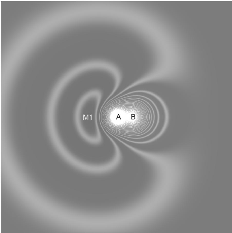
We can clearly see that there is a point M1 near which a second B particle would be stable. This starts to give us an idea of how a pair of electrons could behave in an atomic orbital, in purely inverse-square-law (i.e. electrostatic) terms.
