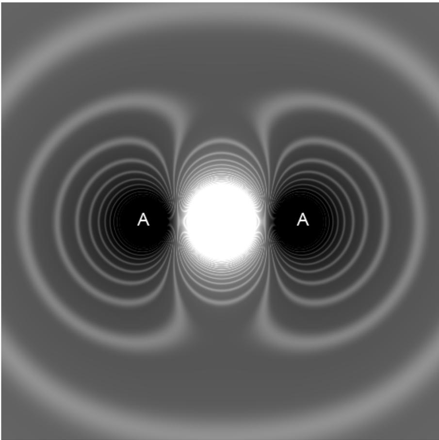
Effectively, a 3rd particle experiences the rotating frame as a repulsion away from the centre point, at the same time as still being gravitationally attracted to the other 2 particles. This is commonly known as Centrifugal Force.
