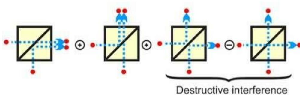
Schematic illustration of the HOM bunching effect of indistinguishable photons in a Beam Splitter.
