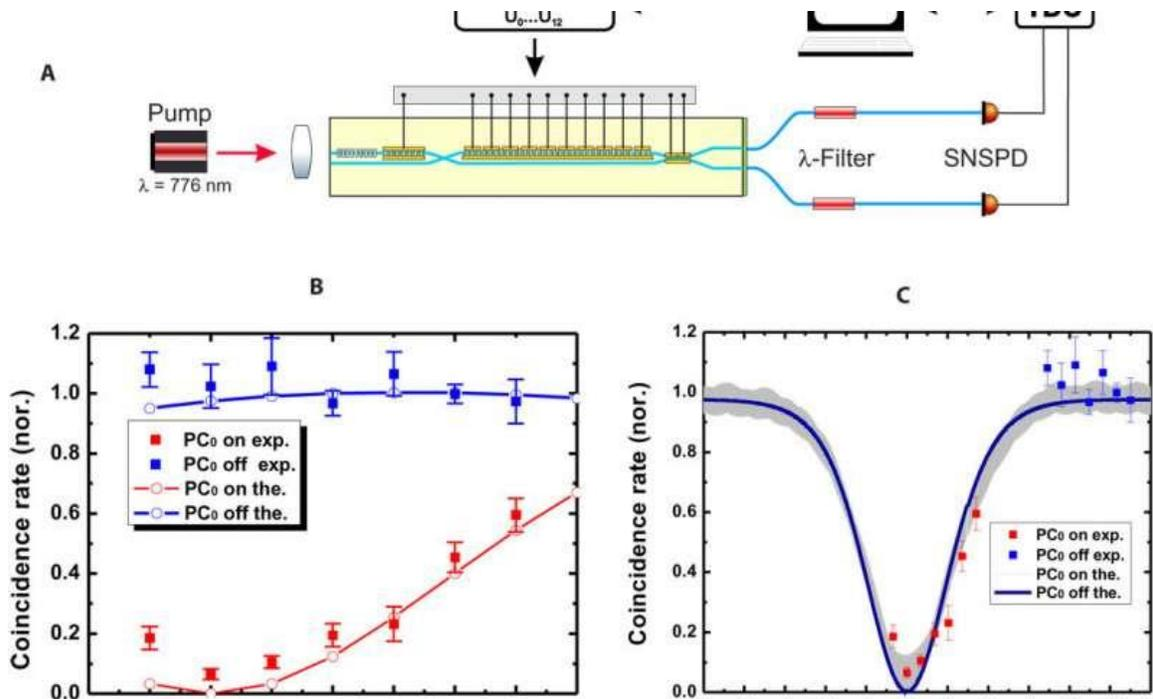
Experimental setup and quantum results. (A) Experimental setup for quantum characterization of the active HOM chip. A tunable narrowband continuous-wave pump laser around 776 nm is coupled into the channel with the PDC source. To avoid ...[more](#)
