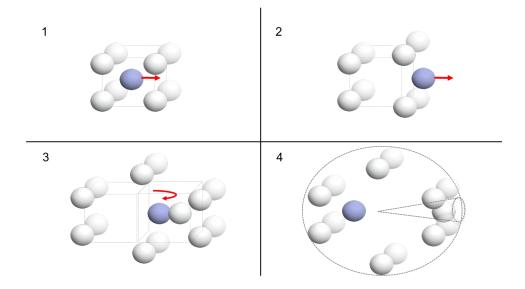
Fig. 2 - Vibration of center granule in body centered cubic unit cell
