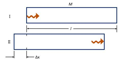
FIG. 1. Einstein's box experiment: An isolated box recoils from its initial position (I) to a final position (II) as a result of a photon traveling from one end of the box to the other.
