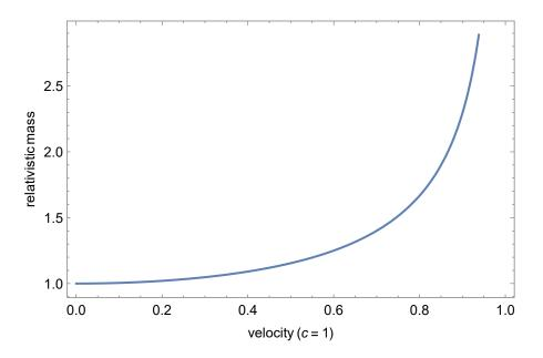
FIG. 2. Dependency between the mass of a body and its velocity. The graph shows how the mass approaches infinity as velocity approaches the speed of light. Thus, it is not possible for an object with mass to reach the speed of light.
