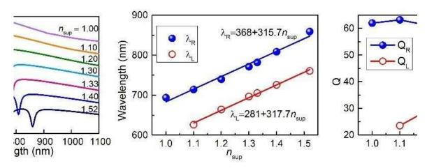
In a less symmetric dielectric environment (that is for smaller nsup), the conventional SLR has a lower quality factor but the novel SLR has a higher quality factor. Credit: SIAT
