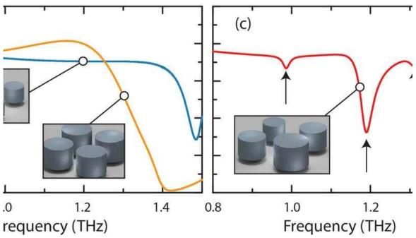
When the frequency responses of dielectric metamaterial setups consisting of four small cylinders (blue) and four large cylinders (orange) are combined into a setup consisting of three small cylinders and one large cylinder (red), the resulting response looks nothing like a straightforward combination of the original two. Credit: Willie Padilla, Duke University
