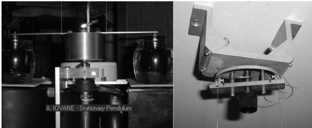
Fig. 1 – Left: the damped bob of the pendulum. Right: the suspension
