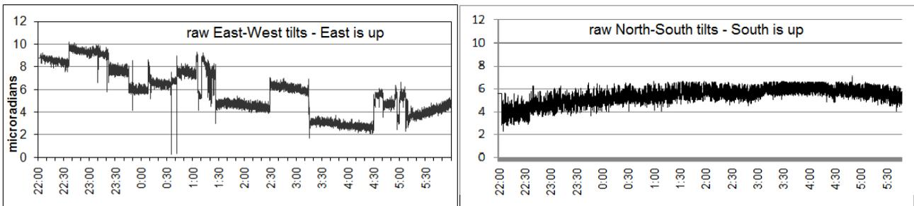
Fig. 11 – Uncorrected 8-hour continuous data around the eclipse.. East-West and North-South
