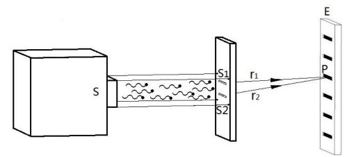
Fig. 3.1 Light beam double-slit interference experiment
