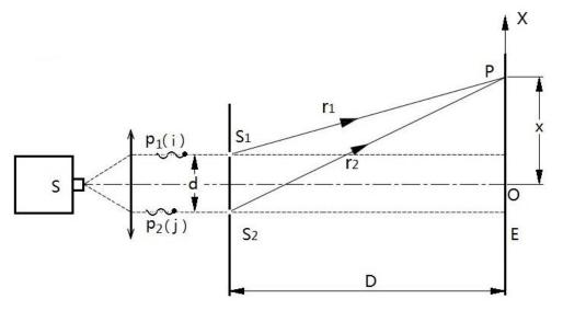
Fig. 3.2 Single photon double-slit interference
