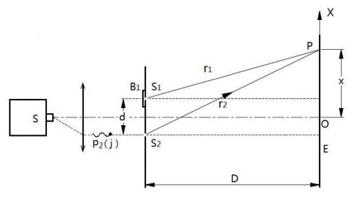
Figure 3.3B Single photon double-slit interference (S1 blocked)
