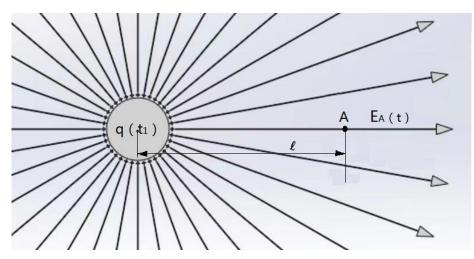
Figure 4.1 Electric field wave excited by periodically varying charge
