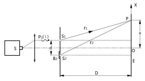
Fig. 3.3A Single photon double-slit interference (S<sub>2</sub> blocked)
