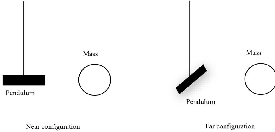
As can be seen from Figure 1, the two methods are consistent with the orientation of the time-of-swing method's device for measuring gravitational constants. Just reduce the attraction ball from symmetrical two to one. In this way, the two angular frequencies of the near configuration and the far configuration of the pendulum are measured, which are  $\omega_n$  and  $\omega_f$
