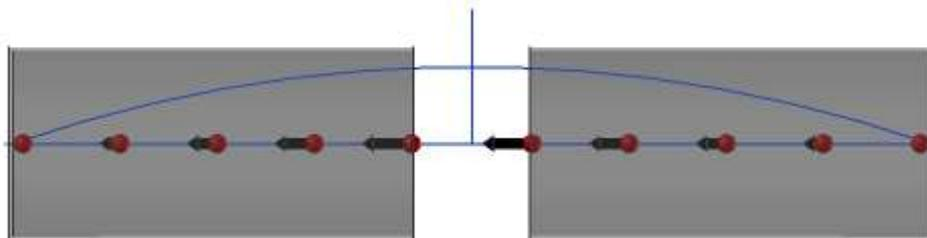
Note that the electrons move to-and-fro along the antenna about fixed positions in the antenna and what we represent on the vertical axis is only their maximum displacement from their fixed points (which is the amplitude of their oscillation). When the electrons move to the right we show their maximum displacement (amplitude) downwards:
