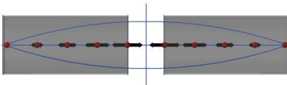
... that shows electrons oscillating backwards and forwards along the antenna and their
