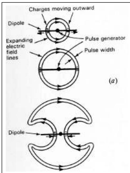
At the next stage [(a) middle] the charges reach the ends of the dipole, are reflected (bounce back) and move inward toward the generator [(a) bottom].
