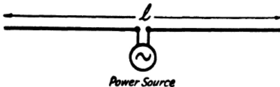
The movement of air particles in the tubes and of the electrons the antenna is oscillatory: they move forwards-backwards (to-and-fro) along the antenna about fixed positions executing simple harmonic motions.
