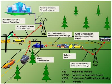
Fig. 2. Communication in vehicular networks.
