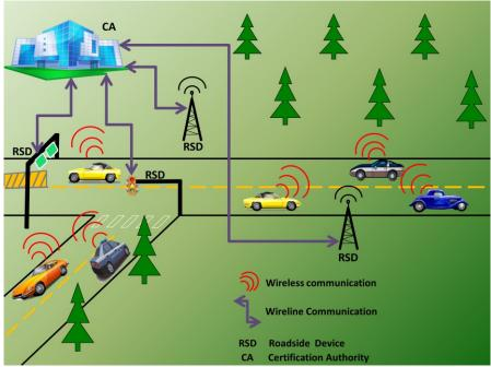
Fig. 1. Vehicular communication network architecture.
