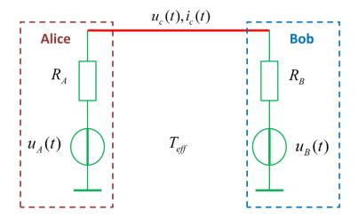
Fig. 3. Illustration of the core Kirchhoff-Law-Johnson-Noise (KLJN) secure key distribution system.
