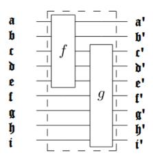
The input lines all carry one qubit each. The gate f operates on the first five lines and then the g gate operates on the last seven lines. The input can be seen as a tensor product multi-qubit of 9 single qubits represented compactly as
